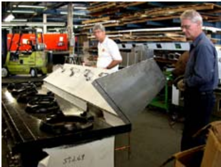
2. Remove sidesplash bolts and lower backsplash
