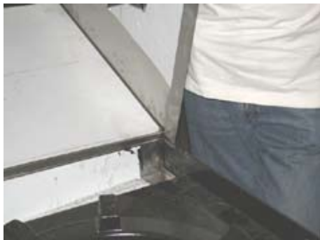
4. Lower backsplash until sidesplash clears gutter
